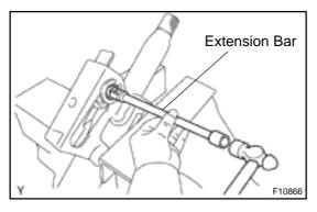
(b) Using an extension bar and a hammer, drive in the bracket spacer.
