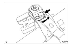
(d) Install the No. 1 support reinforce with the No. 2 tilt lever lock bolt by turning it counterclockwise.
