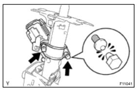
7. INSTALL COLUMN UPPER BRACKET AND COLUMN UPPER CLAMP
