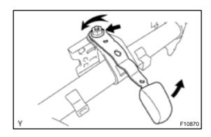
(c) Install the adjusting nut by rotating it counterclockwise in the specified torque so that the locking load (load applied to when a knob is operated) of the tilt lever will be 38-82 N (3.9 -8.4 kgf, 8.5-18.4 lbf).
